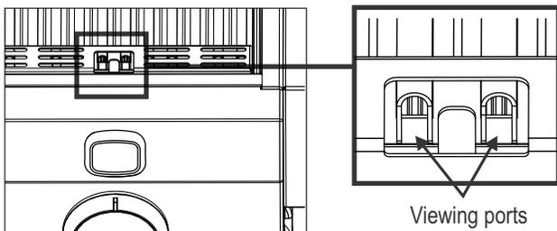
6. If ignition does **NOT** occur in 5 seconds, turn the burner controls to
