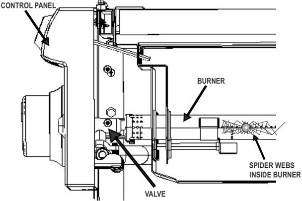
In some areas of the country, spiders or small insects have been known to create "flashback" problems. The spiders spin webs, build nests and lay eggs in the grill's burner tube(s) obstructing the flow of gas to the burner. The backed-up gas can ignite in the burner behind the control panel. This is known as a flashback and it can damage your grill and even cause injury.
