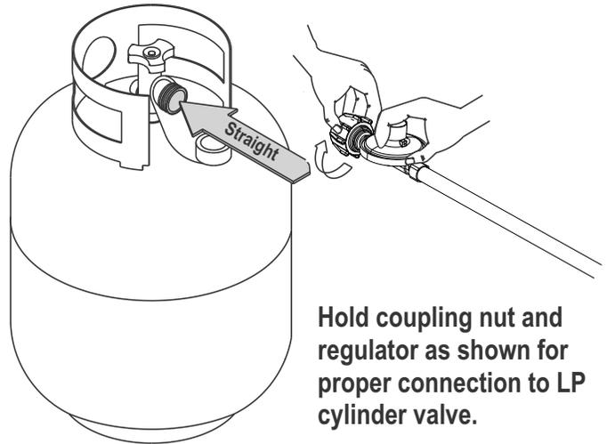
Hold coupling nut and regulator as shown for proper connection to LP cylinder valve.
