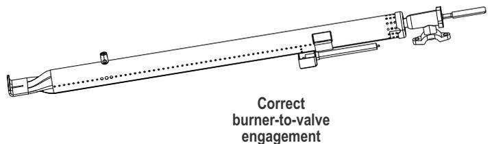
12. Re-attach burners to brackets inside burner box.
