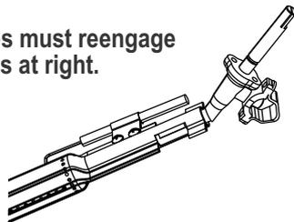
9. Attach electrode to burner.
