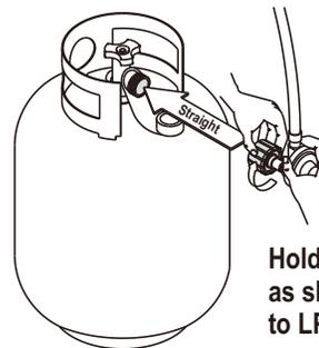
**Hold coupling nut and regulator as shown for proper connection to LP cylinder valve.**
