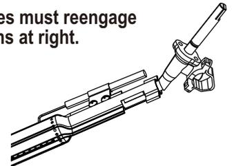
9. Attach electrode to burner.
