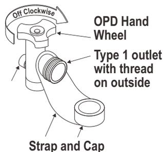
**Do not use a POL transport plug (plastic part with external threads)! It will defeat the safety feature of the valve.**
