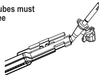
9. Attach electrode to burner.
